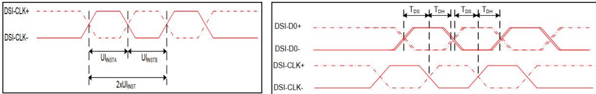
Figure 4 DSI clock channel timing
